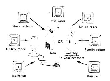
TE: For those who are "heavy sleepers" may not be awakened by flashing lights, vibrators (under bed pillows) can be connected to the switched receptacles.
