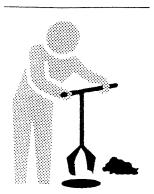
Begin by boring a starter hole 3" to 5" in diameter and 18" to 30" deep. Bore this hole with a hole digger or hand auger.
