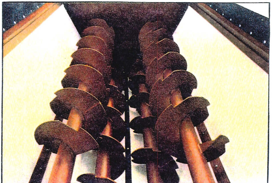
The augers shown in this photograph are typical in a "mixer-feed truck". The augers mix corn, hay and other feed ingredients that are placed directly in the "mixer-feed truck". Consequently, there is no top to the "mixer-feed truck".
