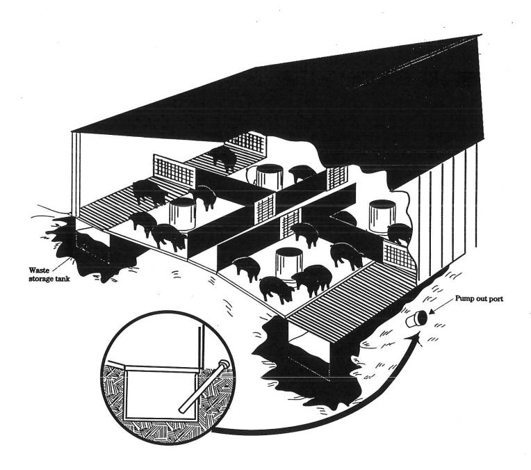
Figure 9-18 Two stage aerobic lagoon system for treatment of waste flushed from swine building
