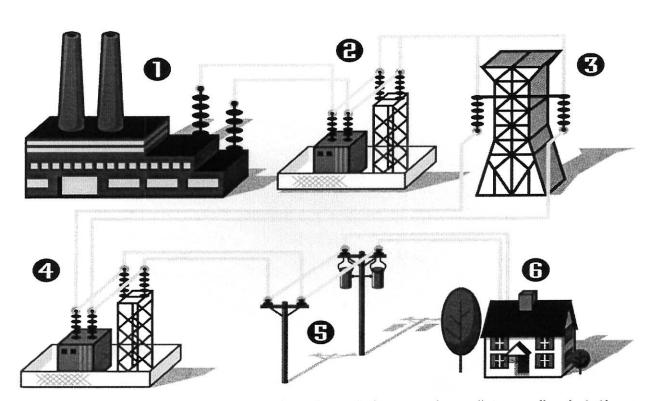
When electricity leaves a power plant (1), its voltage is increased at a "step-up" substation (2). Next, the energy travels along a transmission line to the area where the power is needed (3). Once there, the voltage is decreased, or "stepped-down," at another substation (4), and a distribution power line (5) carries the electricity until it reaches a home or business (6).
