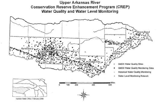
Water levels have been monitored at least annually at numerous locations in the CREP counties. The figure above includes the locations of historical water level measurements in the area. GMD5 obtains water level measurements from 25 wells in the CREP area. Annual measurements are collected from 14 of these wells and quarterly measurements of 11 wells are planned to continue.
