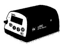
The equipment was set to a oneminute log interval, which averages previous one-second 60 measurements. Sampling was discreet in order not to disturb the occupants' normal behavior. The Sidepak is about 5x4x3 inches and weighs about one pound. For each venue, the first and last minute of logged data were removed because they are averaged with outdoors and entryway air. The remaining data points were averaged to provide an average  $PM_{2.5}$ concentration within the venue.
